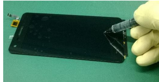
Please don't operate with sharp stick such as pens 请不要用尖锐的物体来操作，例如用笔尖
