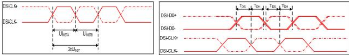
Figure 4 DSI clock channel timing
